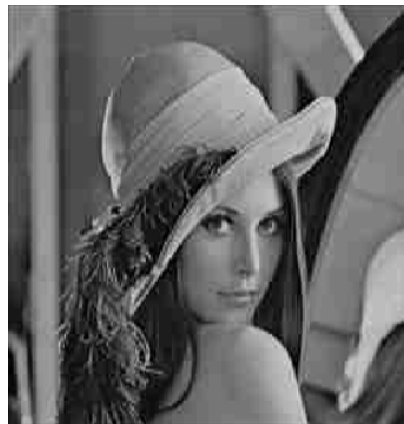
Figure 8: Lena (Spline with 1 level of decomposition + JPEG compression + Preprocessing) coded at 0.14 bpp and PSNR = 28.2 dB
